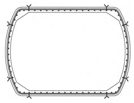
**Canopy Cover Tie Locations:** Working on your boat or on a work table center your canopy cover on the frame using the 8 ties provided as shown. figure # 4
